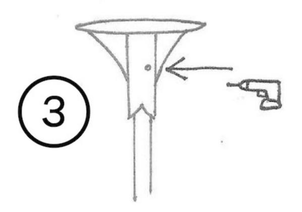
Fit birdhouse on base. Check for equal overhang. Secure through pilot holes.
